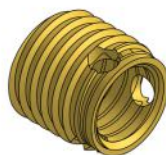
TYPE 8 : Self-tapping with 3 cutting bores, thin wall
